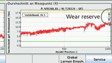
Spindle 2 Sufficient wear reserve
